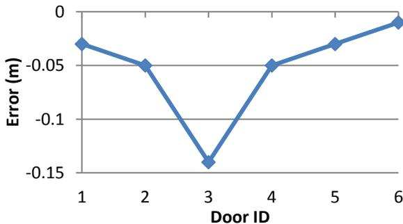
Figure 4. Errors for the door width measurements
