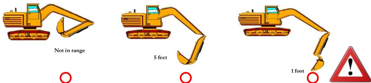
Figure 5 In-cab collision avoidance output for operator
