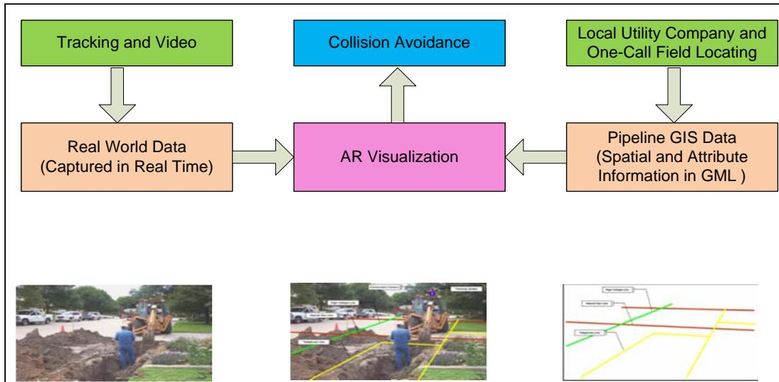
Figure 3 Data Flow for Collision Avoidance System Using Augmented Reality
