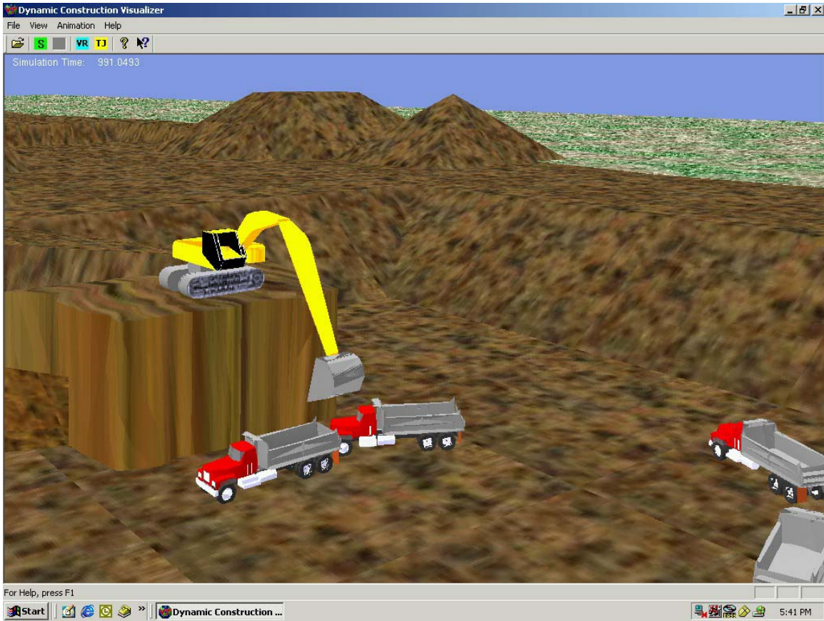
Figure 5. Modeling Flaw: Rear-end Collision at the Main Loading Area
