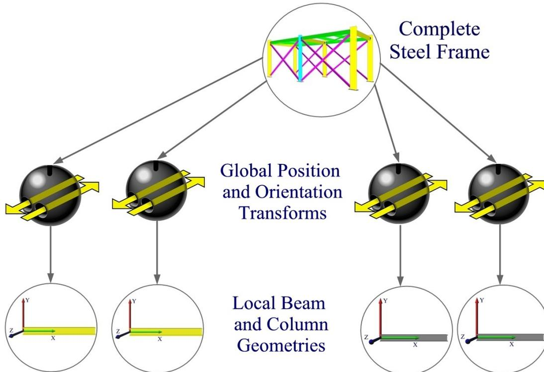
Figure 3: Local VRML Geometry Nodes with Collapsed Transformations
