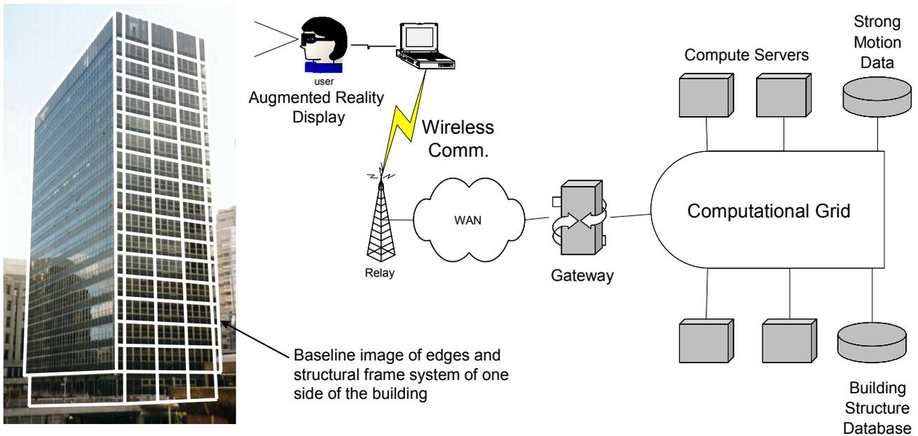
**Figure 1: Overall Architecture of the New Damage Reconnaissance Methodology.**
