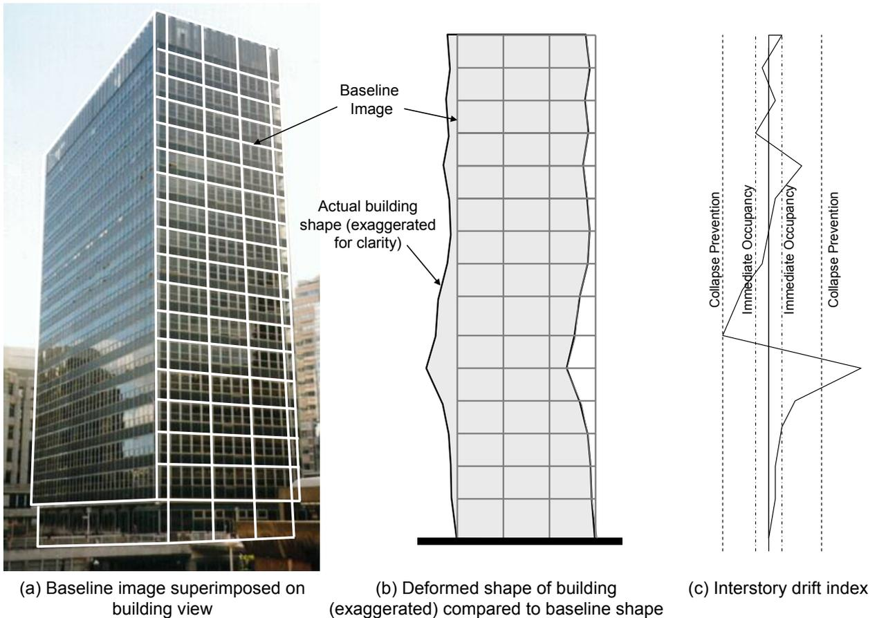
**Figure 2: Computation of Residual Interstory Drift Ratios (IDRs) After a Seismic Event.**
