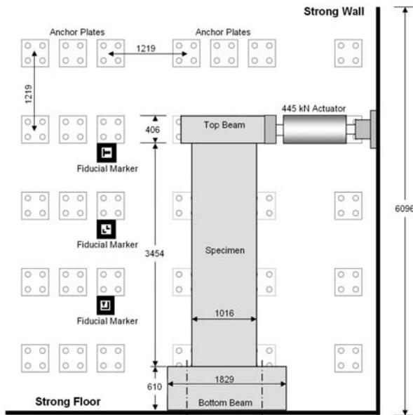
**Figure 2:** Experimental Setup in the UM-SEL (all dimensions in mm)
