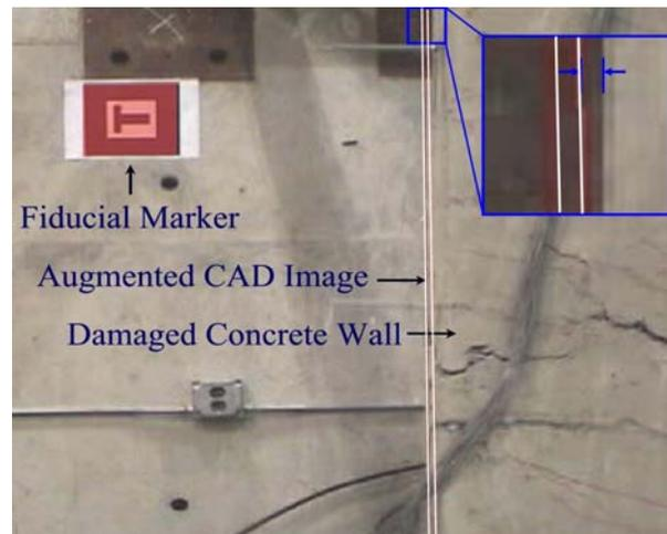
**Figure 4:** Observed Displacement (zoomed for clarity) Between Registered Augmented CAD Image and Real Damaged Concrete Wall Specimen
