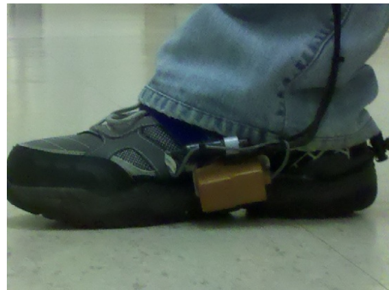
Figure 2: Small sized nIMU used for this research
