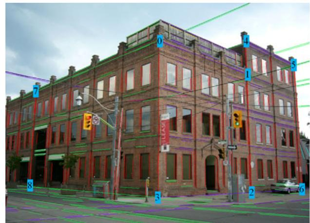
**Fig. 11** LSD and J-linkage output—the first three classes are drawn in red, green, and purple, respectively (color figure online)
