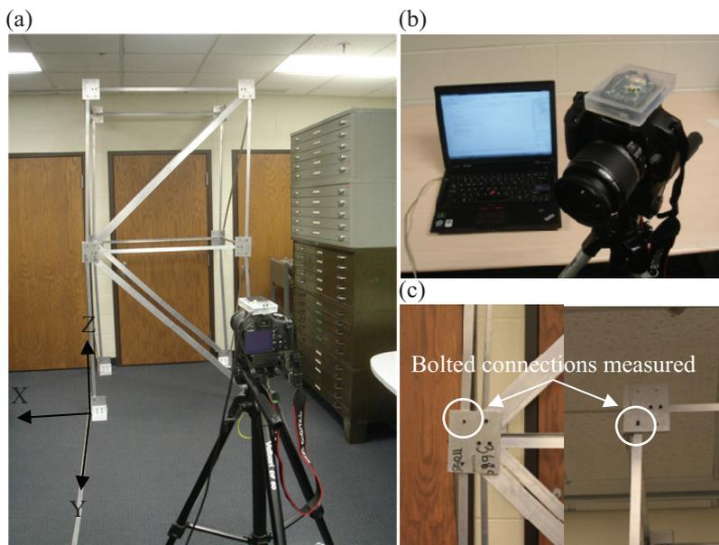
Fig. 8: (a) Experiment setup overview, (2) customized compass attached on the camera, and (3) bolted connections denoting positions of two inspected floors
