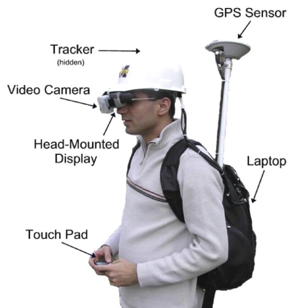
Fig. 1. Overview of the developed AR hardware framework.
