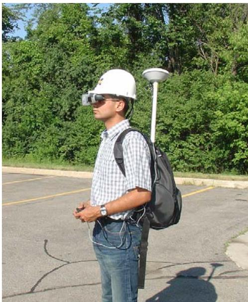
**Figure 4:** Profile of a user equipped with the mobile computing apparatus designed in this research
