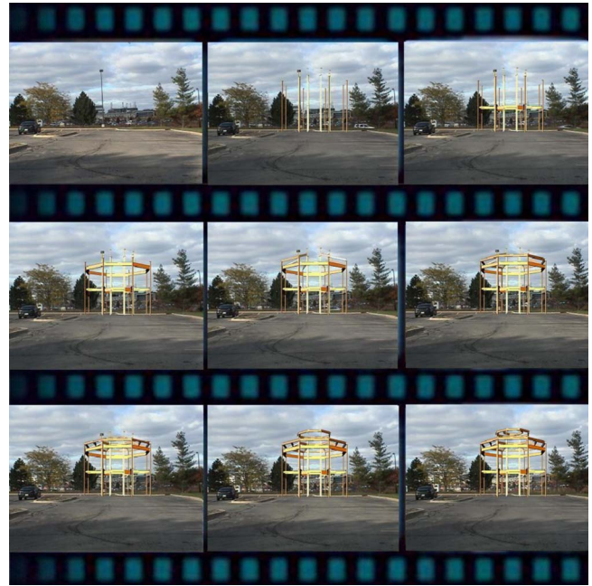
Fig. 14. Graphical augmented reality simulation of a 4D CAD model
