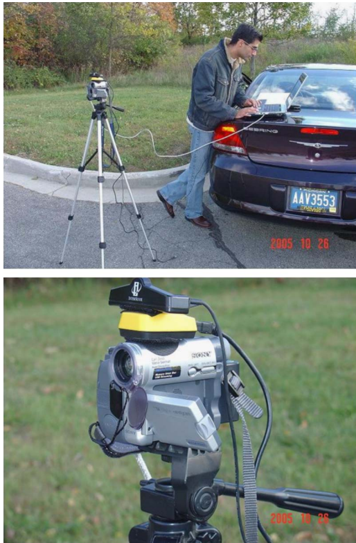
Fig. 11. Hardware setup of UM-AR-GPS-ROVER
