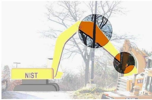
Fig. 15. Dynamic occlusion problem in outdoor augmented reality
