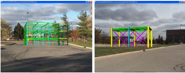
Fig. 13. Structural steel frames registered in outdoor augmented reality
