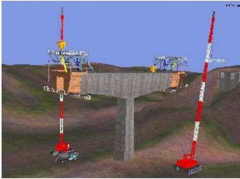
Virtual Reality Bridge Construction Model
