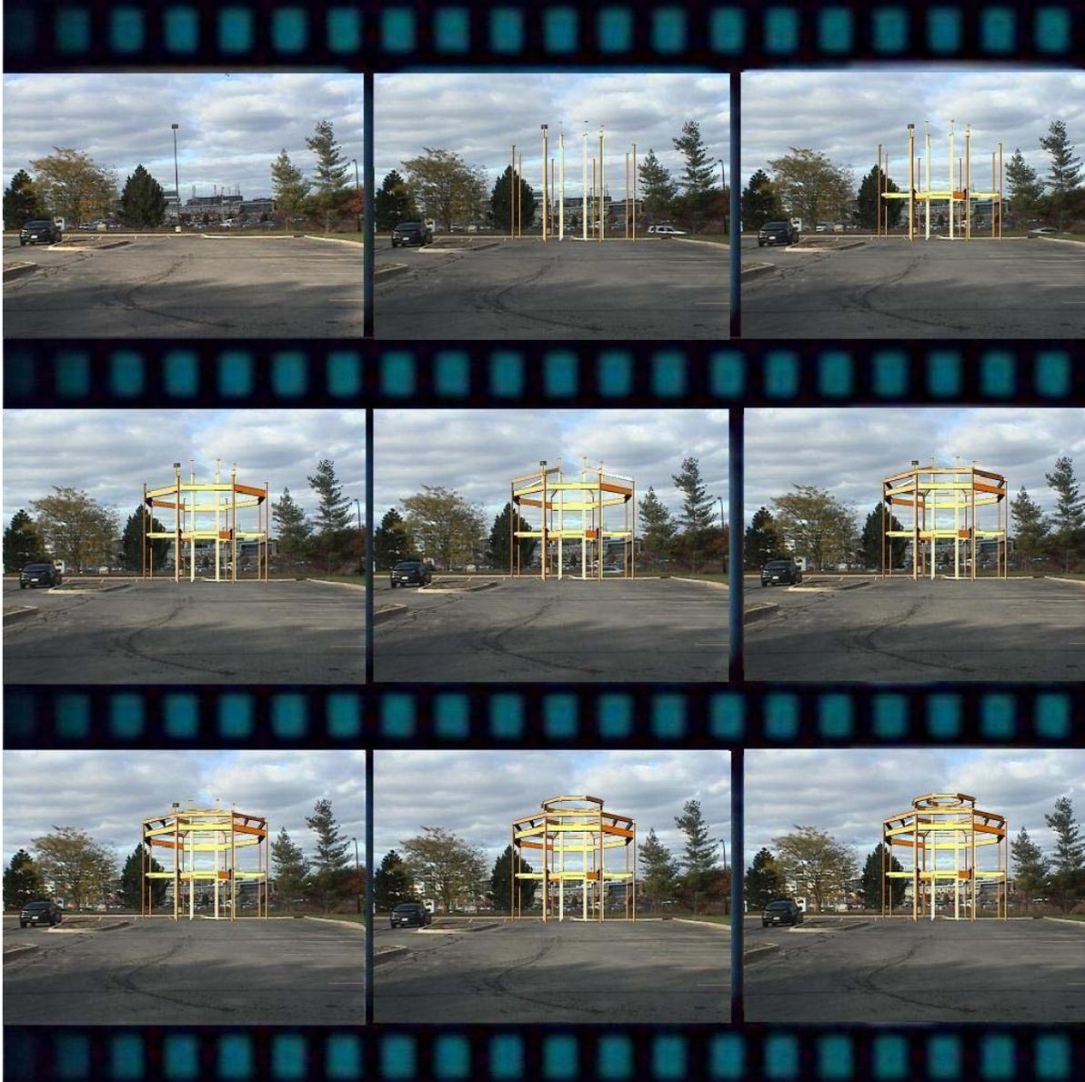
Figure 5: Graphical Augmented Reality Simulation of a 4D CAD Model
