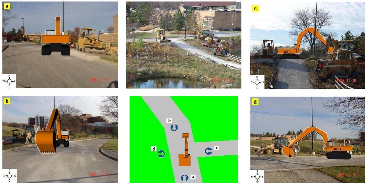
Figure 3: Concept of Accurate Outdoor Augmented Reality Registration
