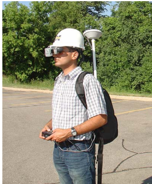
Figure 5: Observer Equipped with Position and Orientation Tracking Devices
