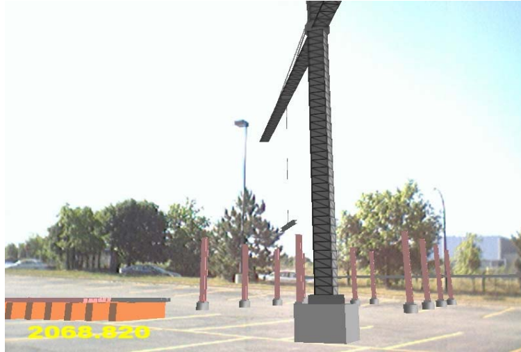
Figure 6 – An Augmented Reality Animation of a Steel Erection Operation
