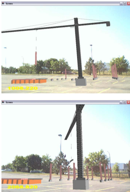
Fig. 15. Steel erection operations (ARVISCOPE) with user's global position change
