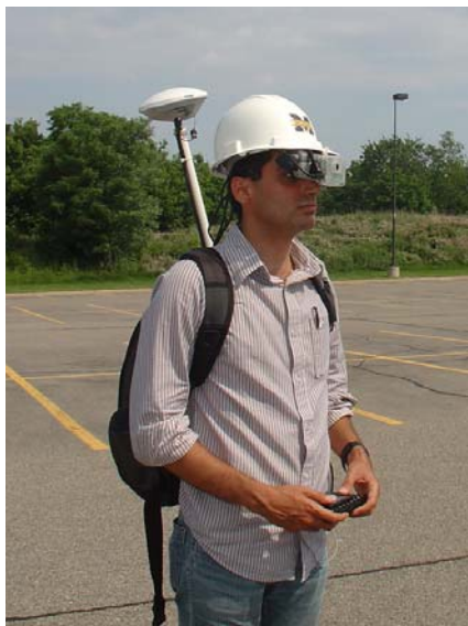
Figure 4: Profile of a user equipped with UM-AR-GPS-ROVER mobile AR apparatus
