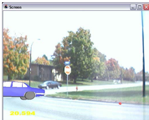
Figure 10: Virtual car is crossing the intersection while the real car is waiting
