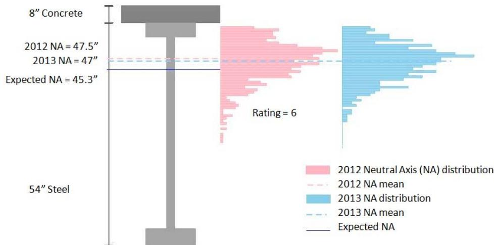
**Figure 4. Movement of the composite action neutral axis between 2012 and 2013 as observed in the second girder (from the south-west) of the middle span in the CSB**
