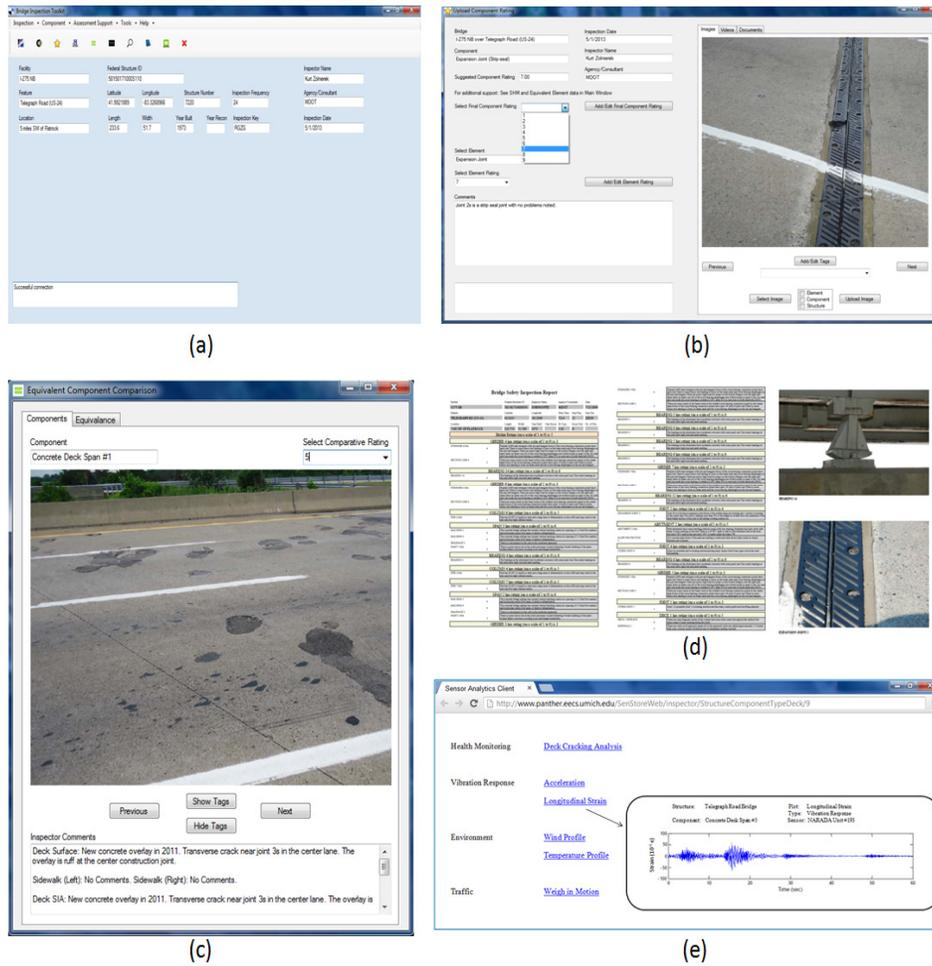
**Figure 3. (a) The Graphical user interface of the BIT and the (b) rate component, (c) equivalent component comparison, (d) generate report, and (e) SHM analysis functionality available in the BIT**
