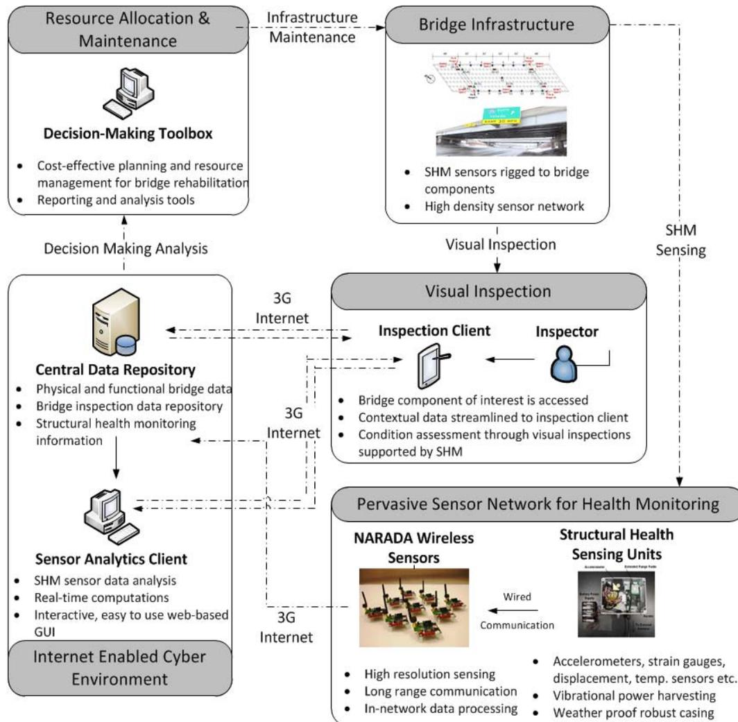
**Figure 1. Architecture of the SHM-integrated bridge inspection solution**
