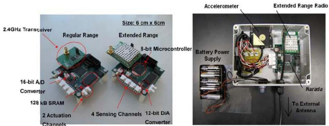
**Figure 2: Narada wireless node (left) and a pre-assembled sensing unit (right)**
