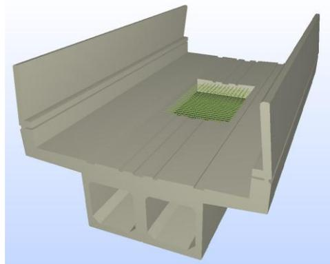
**Figure 8: BIM model of the bridge deck with the embedded rebar cage (green) displayed in an IFC viewer.**
