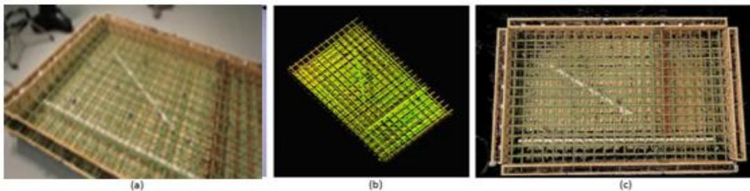
**Figure 2: The point cloud models of (a) the rebar cage as developed from (b) laser scanning and (c) image based 3D reconstruction [Saidi, K., et al., 2011].**
