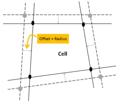
**Figure 3: Extracting the quadrilateral cells in the rebar mapping algorithm. The dashed lines represent the projections of the center lines of the cylinder and the solid lines are the offsets equal to the corresponding radii.**
