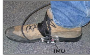
Figure 1. RTK accuracy (Trimble, 2005: AgGPS 332). Figure 2. Small sized nIMU used for this research.
